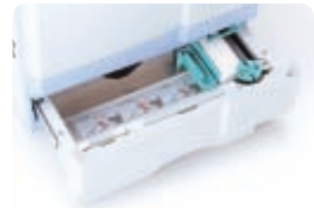
Card hopper holds up to 300 cards(0.76mm)
